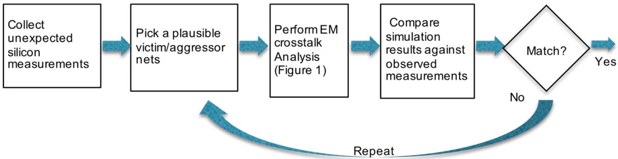
**Figure 2: Using EM Crosstalk Analysis to Debug Silicon Issues**
