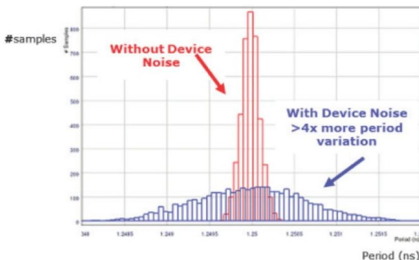
Fig 1: Device noise impact on PLL jitter. Source Mentor.
